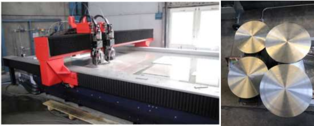
Left: Water cutting of blanks, right: manufactured platforms
